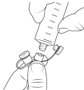
ENFit® syringe twisting into an ENFit® tube
